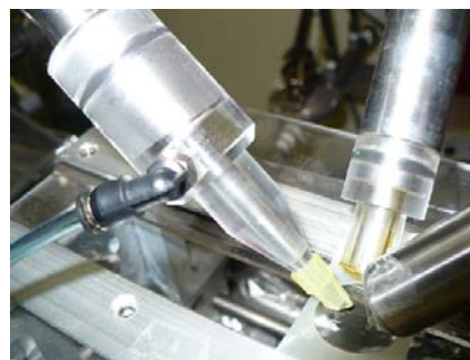
Fig 11. Photograph of cap attached at the tip of the Detector No. 2
