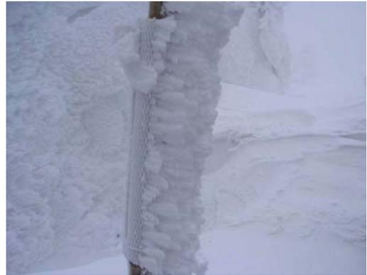
Fig. 2 Photograph of rime adhered to the Teflon® net. The photograph was taken 16 February 2004.
